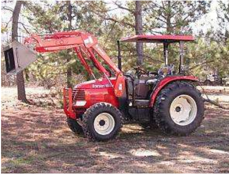
New Branson 5530R – 55 HP, 4 WD Tractor with loader, 24 Sp, Synchronized Transmission with shuttle shift, Ind PTO, Loader lift capacity 3100 lbs, 4 yr. limited warranty. Call for price.
