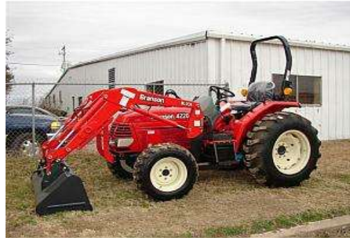
New Branson Tractor 4220i – 42 HP 4WD Tractor/Loader, 12 sp synchronesh transmission with shuttle shift Ind PTO load capacity 2200 pds, 4 yr. limited warranty. Call for price.
